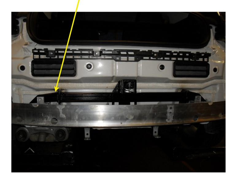
**Step 9.** Re-install bumper fascia on to vehicle. Push bumper fascia until all plastic clips lock into place on rear fascia guides. Replace all fasteners removed in previous steps.
