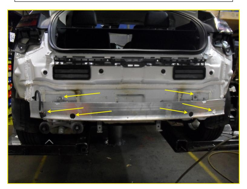
Step 8. Position trailer hitch onto six studs. Notice the orientation of the hole pattern. This hitch can only go on one way. Place the bumper impact bar back over the trailer hitch. Hand tighten bumper impact bar nuts to ease the installation of the bumper impact bar. Re-torque bumper impact bar nuts to 38ft lbs.
