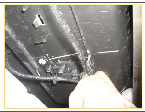
**Step 4.** Starting with the passenger side rear fender well, remove the torx fasteners from the bumper fascia. There are 4 fasteners total. Use the T20 torx bit to remove these fasteners. Once completed, repeat for drivers side.
